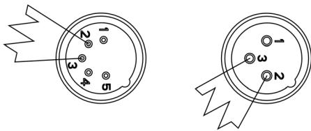
A DMX512 terminator reduces signal errors, avoiding most signal reflection interference. Connect PIN 2 (DMX-) and PIN 3 (DMX+) of the last fixture in series with a 120 Ohm, 1/4 W Resistor to terminate the DMX512.
